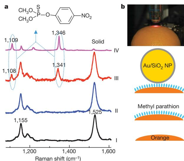
**Figure 4** | *In situ* inspection of pesticide residues on food/fruit. **a**, Normal Raman spectra on fresh citrus fruits. Curve I, with clean pericarps; curve II, contaminated by parathion. Curve III, SHINERS spectrum of contaminated orange modified by Au/SiO<sub>2</sub> nanoparticles. Curve IV, Raman spectrum of solid methyl parathion. Laser power on the sample was 0.5 mW, and the collected times were 30 s. **b**, Schematic of the SHINERS experiment.
